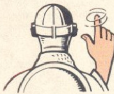
6. One Finger, Circular Motion Check Your Tachometer and Throttle Setting
