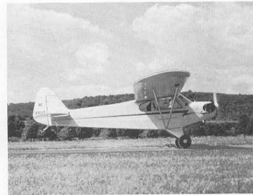
18. With tail up, in level flight position, ready to leave the ground.
