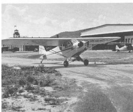
15. Observe the windsock and S-taxi to the runway. Always take off and land INTO the wind. Do not taxi faster than normal walking speed. Look around and ahead constantly for other aircraft.
