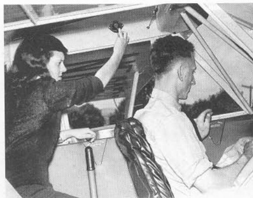
16. Near end of runway stop, apply brakes, advance throttle to 1400 RPM and check the magnetos with the tachometer. Check for other aircraft landing or taking off. If clear, proceed to position on runway.
