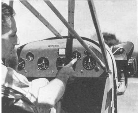
13. Check oil pressure gauge for normal reading.
